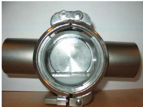
Figure 1. Illustrates how a spherical valve body or instrument casing can cause insufficient drainage through wrong installation. There will always be liquid at the bottom.
